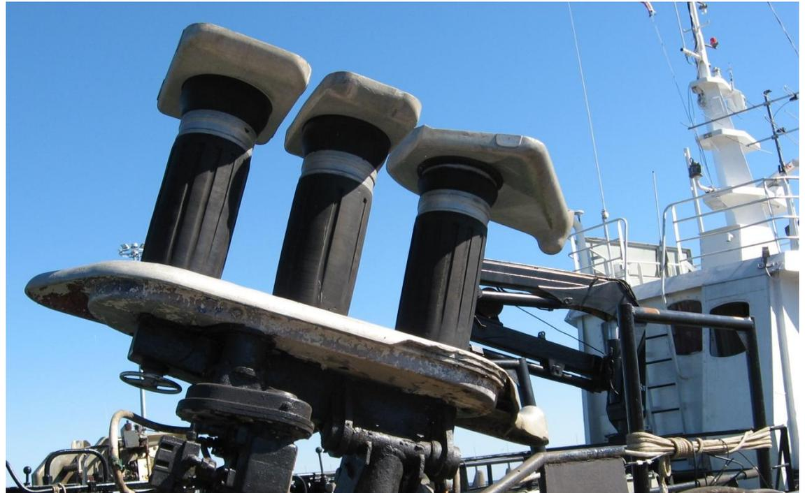
**Fig. 2** TRIPLEX: traction drums cover with rubber
