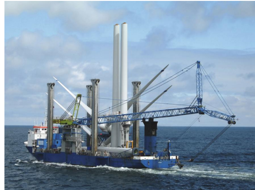
Jackup vessel loaded with wind mills. (source: earthandindustries.com)
